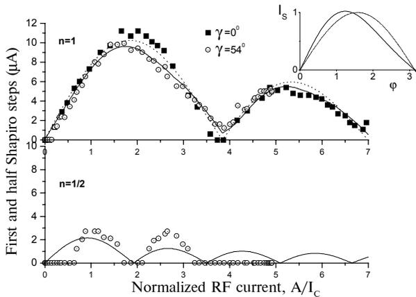
Fig.3. Normalized RF current dependence of the first and half Shapiro steps for two junctions  $\gamma=0$  (squares), and  $\gamma=54^\circ$  (open circles). Dashed and solid lines show the calculated curves for  $\delta=0$  and  $\delta=0.2$  correspondingly. The current-phase relations  $I_s(\phi)$  for these two cases are shown in inset.
