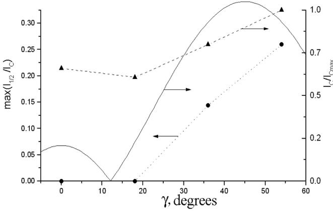
Fig.4. Dependencies of the maximum of the Shapiro subharmonic step and the critical current density on the angle of the deviation of the current direction from the normal. The solid curve gives the critical current  $I_c$  of JJ as a function of the angle of asymmetry of the bicrystal interface [13]
