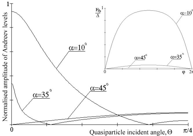
Fig.5. Maximum of Andreev's levels in  $D_\alpha ID_\alpha$  junctions over  $\varphi$  for several  $\alpha$ . The inset shows phase dependence of Andreev's levels in  $D_\alpha ID_\alpha$  junction for several  $\alpha$ ,  $\theta = \pi/10$ .
