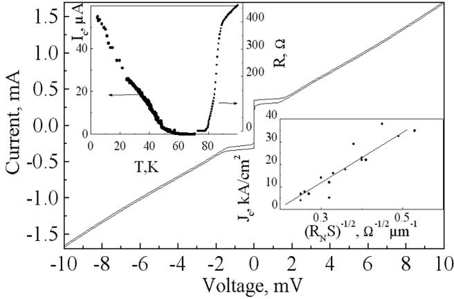
Fig.2. The I-V curve at  $T=4.2\text{K}$  for a typical bicrystal junction. Temperature dependence of the resistance  $R(T)$  and critical current  $I_c(T)$  are shown in the left inset. Dependence of the critical current density  $J_c$  vs. inverse square root of characteristics interface resistance  $(R_N S)^{-1/2}$  at  $T=4.2\text{K}$  is shown on right inset.
