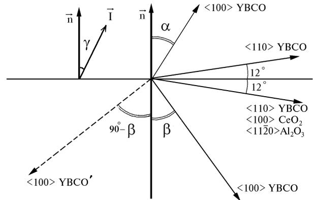
Fig.1. Crystallographic axes orientations of  $\text{CeO}_2$  and YBCO films in sapphire bicrystal junction with  $\alpha = 33^\circ$ ,  $\beta = -33^\circ$  ( $D_{33}ID_{33}$ ). The domain of the film with the direction  $\langle 100 \rangle \text{YBCO}'$  misoriented on the angle  $\beta' = 90^\circ - \beta$  is the twin to YBCO.
