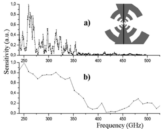
Fig. 3. Amplitude-frequency characteristics for a log-periodic antenna with a BJJ on sapphire at  $T = 20$  K. (a) a metal (platinum) antenna was used, (b) all HTSC sample, evaluated by use of Fourier Transform Spectrometer.
