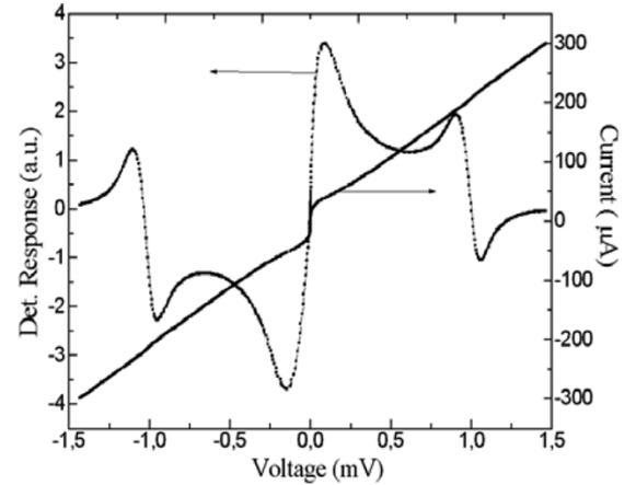
Fig. 2. Detector response of bicrystal Josephson junction on  $\text{NdGaO}_3$  substrate for  $T = 80$  K. An external 500 GHz radiation was applied. The response has two distinct features: first is the wideband response at low voltages and second is the frequency selective response at voltage  $V = hf_e/(2e)$ .
