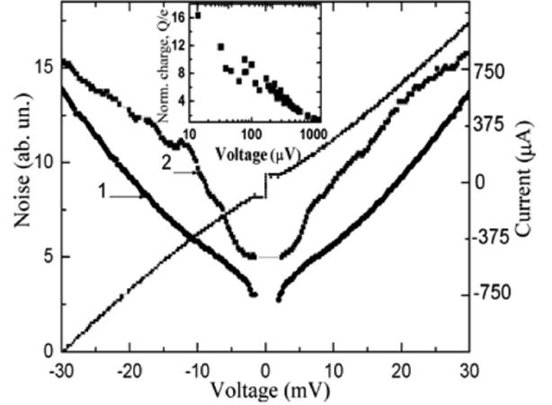
Fig. 5. The  $I$ - $V$  curve and noise power  $P_N(V)$  in the 1–2 GHz frequency band (curve 1), and the 3–300 kHz band (curve 2) for a BJJ on sapphire substrate at  $T = 4.2$  K. Inset: noise/current ratio in terms of effective transferred charge  $q(V)$  for bias voltages  $V < 1$  mV.
