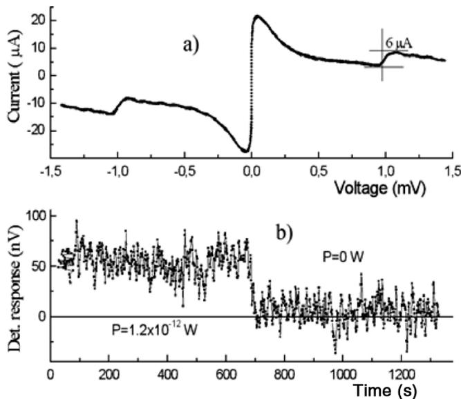
Fig. 6. Calibration of absorbed power and radiometric measurements at  $f = 500$  GHz,  $T = 80$  K a)—Josephson part of reduced  $IV$ -curve ( $I(V) - I \cdot (R_N)$ ) with Shapiro steps which allow us to estimate the power absorbed by the junction at high signal levels. b)—noise trace at low signal-to-noise ratio for known absorbed power. The NEP is estimated to  $6 \cdot 10^{-13} \text{ W/Hz}^{1/2}$ .
