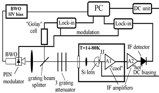
Fig. 1. Block diagram of set-up. The BWO is a submm wave source  $f = 220\text{--}550$  GHz or  $800\text{--}900$  GHz. The PIN modulator is specially designed for the THz frequency range. The beam splitter is made from a metallic net. For simplicity the set of Teflon lenses is shown as one. The Golay cell is a submm wave detector. The Si hemispherical lens has diameter  $d = 12$  mm and extension 3 mm. The JJ indicates the substrate with the BJJ and the integrated antenna.
