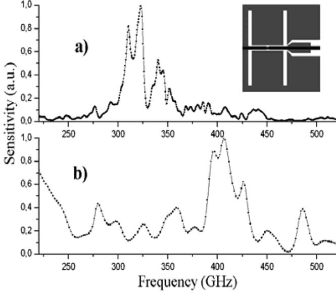
Fig. 4. Amplitude-frequency characteristics for double-slot line antenna designed for 300 GHz (a) and 400 GHz (b). Resonance peaks with quality factor  $Q = 6$  are clearly observed.
