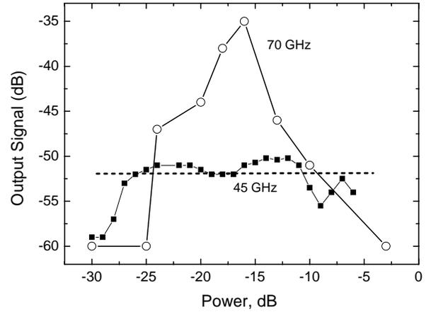
Fig. 2. Output signal measured in 1-2 GHz frequency band under microwave power  $P$  at 45 GHz (black symbols) and 70 GHz (open symbols). Dash line shows saturation level for frequency mixing.
