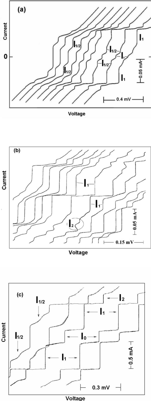
Fig. 1. Families of I-V curves under microwave irradiation  $f=45$  GHz (a, b) and  $f=70$  GHz (c). Critical current  $I_0$ , integer  $I_1$ ,  $I_2$  and half-integer  $I_{1/2}$  Shapiro steps are indicated. (b):  $n=2$  Shapiro step distortion is pointed by circle. (c): chaotic noise rise corresponds to the jerks on  $I_{1/2}$  steps. All curves are shifted by voltage
