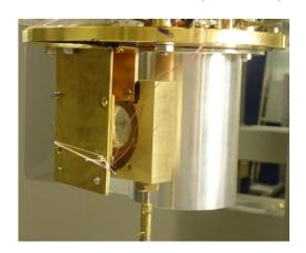
View of the experimental setup mounted in the cryostat. In the photo from left to right: fast black body, interferometer, and bolometer placed inside the aluminium radiation shield. Black body holder, interferometer and radiation shield are mounted on a 2.8 K stage of pulse tube refrigerator, and bolometer attached to 280 mK stage of He<sup>3</sup> sorption cooler.
