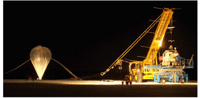
Fig. 5. TELIS-MIPAS launch at Esrange, Sweden; March 2009. Balloon size: 400 000 m 3 ; Payload weight: 1 200 kg.
