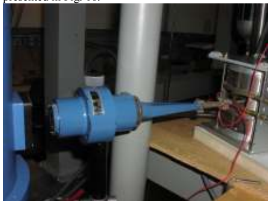
Fig. 15. The backward wave oscillator (to the right), the polarisation grid attenuator (in the center), and the optical window of He3 cryostat (to the left) in the experiment to measure the dynamic range of the bolometer.
