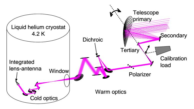
Wire grid polarizer and dichroic plate are used to separate this receiver from the two other frequency channels (not shown). The cold optics and mixer element are located inside the cryostat at the ambient temperature 4.2 K
