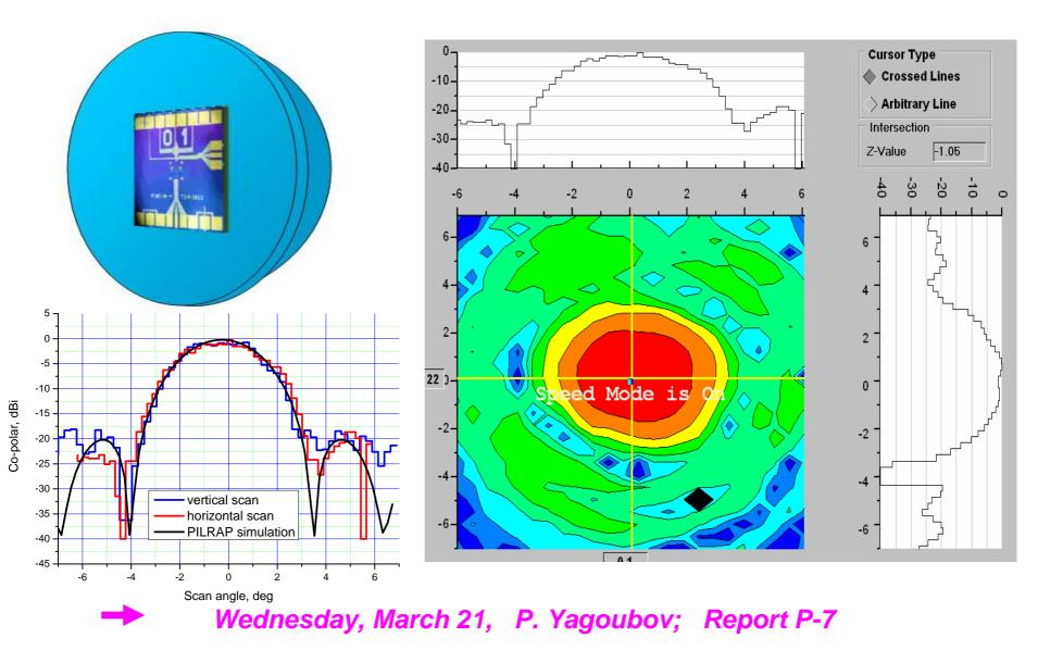
Amplitude and phase APB of the SIR with cold optics
