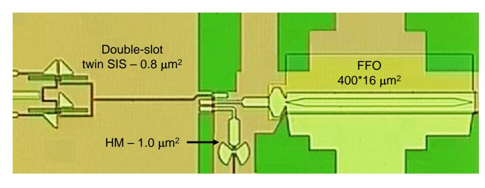
Nb-AIN-NbN or Nb-AIOx-Nb;  $Jc = 5 - 10 \text{ kA/cm}^2$
