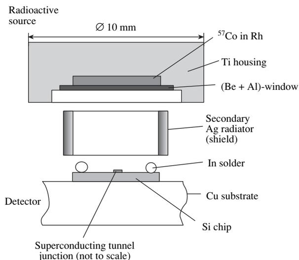
Fig. 1. Geometry of the experiments on fluorescence excitation and detection.
