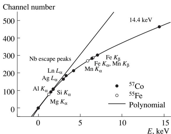
Fig. 4. Energy dependence of the detector's response.
