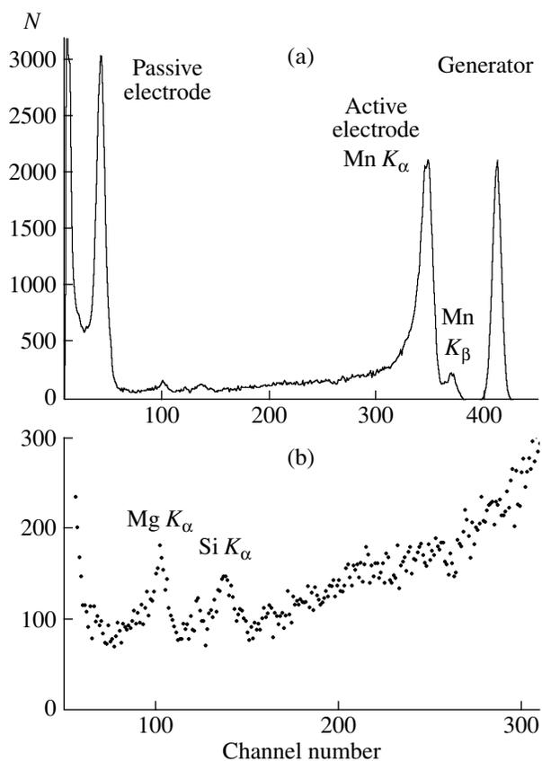
**Fig. 3.** Pulse-height spectrum arising during irradiation of a detector with photons from a  $^{55}\text{Fe}$  source. Different portions of the spectrum are represented at different scales.
