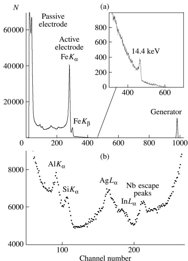
Fig. 2. Pulse-height spectrum arising during irradiation of a detector with radiation photons from a Mössbauer  $^{57}\text{Co}$  source. Different portions of the spectrum are represented at different scales.
