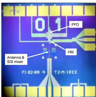
Figure 1. Photo of the SIR chip. Antenna coupled SIS mixer, FFO and HM for FFO phase locking are located on a  $4 \times 4 \text{ mm}^2$  chip. FFO, SIS, and HM are connected with microstrip transmission lines, which contain a number of RF-coupling and dc-blocking elements. The SIS mixer and FFO are provided with local magnetic fields via integrated control lines.
