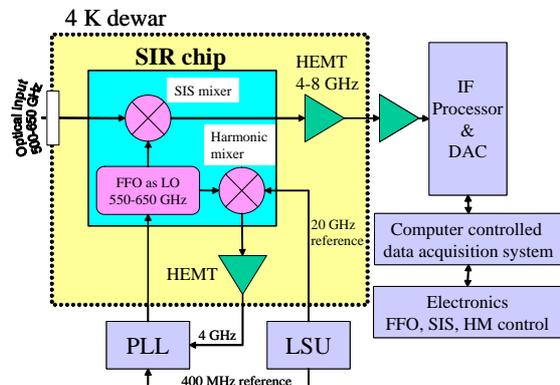
Figure 2. Schematics of the FFO stabilization circuit. FFO frequency is mixed in HM with the harmonic of 19-21 GHz reference. The mixing product is amplified, downconverted and compared with the 400 MHz reference in the PLL. The phase difference signal generated by PLL is used to feedback the FFO control line.
