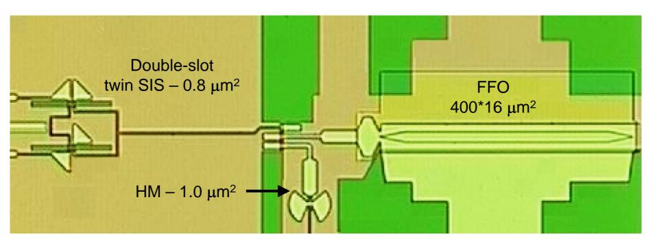
$4 \times 4 \times 0.5 \text{ mm}^3$  (Si); Nb-AlOx-Nb; Jc = 5 - 8 kA/cm<sup>2</sup> Optionally: SIS - Jc = 8 kA/cm<sup>2</sup>; FFO + HM = 4 kA/cm<sup>2</sup>
