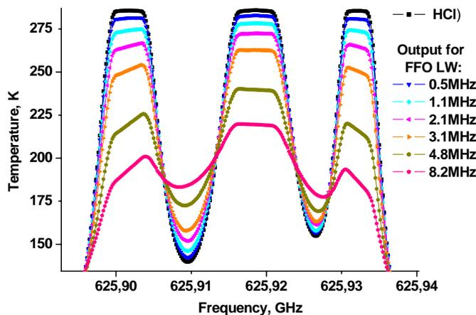
Fig. 6. The form of the output spectra at conversion of the HCl line for phase locked FFO with various free-running linewidth compared to the ‘‘ideal’’ spectrum (when LO spectrum is a  $\delta$ -function).
