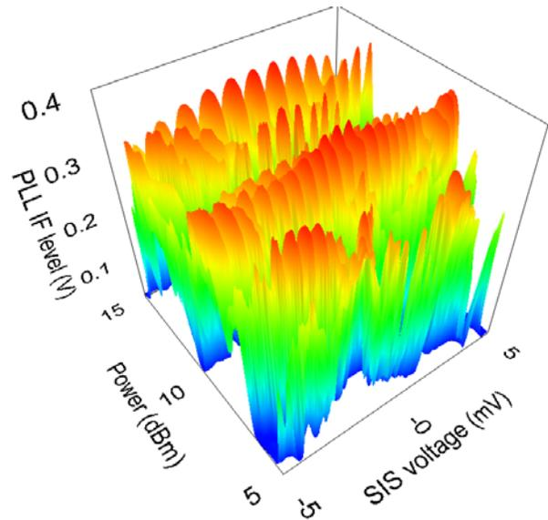
Fig. 3. 3-D diagram for HM operational parameters measured by PC controlled PLL. The level of IF-out PLL signal is represented by color scale; note that normal PL operation is possible at IF levels larger than 250 mV.
