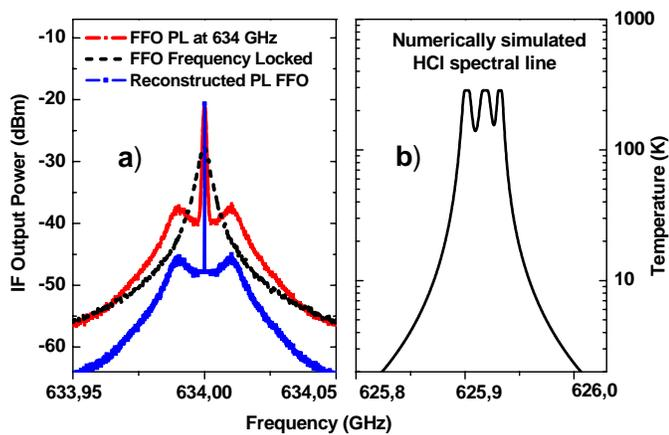
Fig. 5. a) Spectra of the phase-locked and frequency locked FFO; reconstructed spectra: of the PL FFO used for calculations is also shown. b) Computer-simulated spectrum of one of HCl lines.
