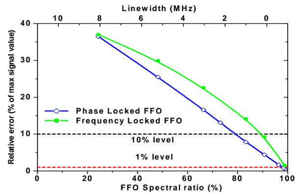
Fig. 7. Relative error of conversion of the HCl line for phase locked and frequency locked FFO. Appropriate linewidth scale is given at the top.
