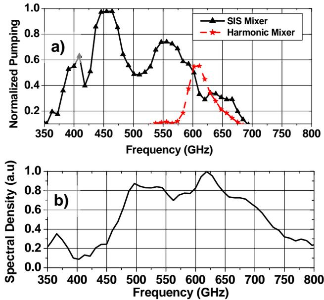
Fig. 2. Frequency characteristics of new SIR chip: a) Pumping current of SIS and HM at a certain frequency normalized at the current rise at the gap voltage for SIS and HM accordingly ( $I_g$  SIS = 100  $\mu$ A,  $I_g$  HM = 172  $\mu$ A). b) FTS data of the double-dipole twin SIS mixer. A dip at 560 GHz corresponds to absorption line of water.
