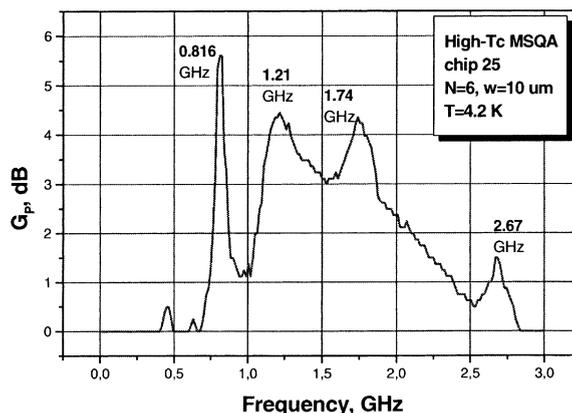
Fig. 4. Measured power gain of the high- $T_c$  dc SQUID RF amplifier.
