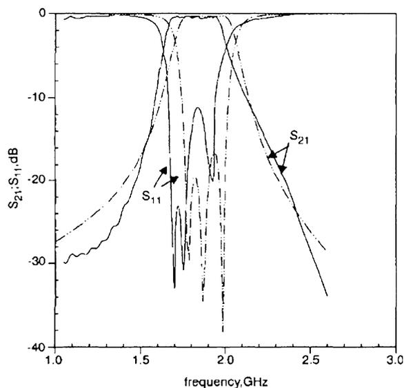
Fig. 2. Frequency characteristics of a three-pole co-planar CPW filter at 77 K.
