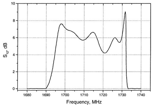
Fig. 7. Frequency characteristic of SQA and band-pass filter combination at  $T = 35$  K.
