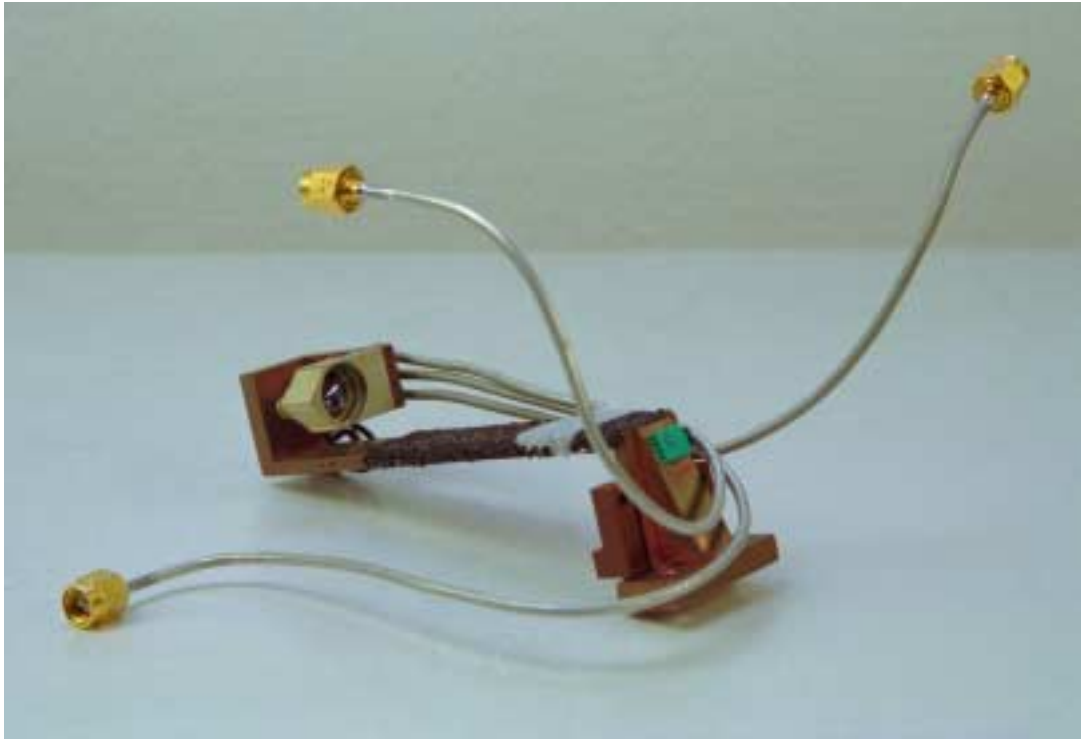
Fig. 2 General view of PLL SIR pixel. The mount of the imaging array is adapted. Three cables are connected to i) SIS mixer for IF/dc-bias, ii) FFO for PLL feedback, iii) harmonic SIS mixer for reference/PLL-IF/dc-bias.
