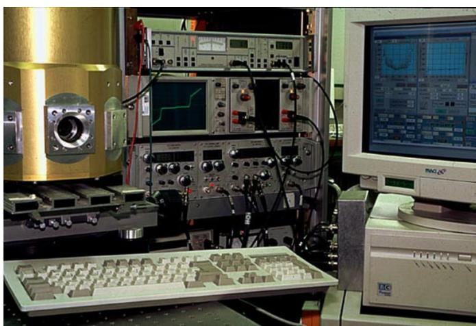
**Figure 11.** Photo of the experimental set-up controlled with the IRTECON system: quasi-optical cryostat on the left, bias supply unit in the centre (in the background) and data display on the right.
