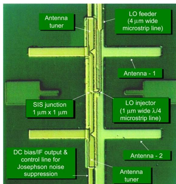
**Figure 8.** Microphotograph of a double-dipole antenna SIS mixer of the integrated receiver. Microstrip tuners for the antenna and a feeder of the local oscillator are shown. The field of view is about  $100 \mu\text{m}$  by  $150 \mu\text{m}$ .
