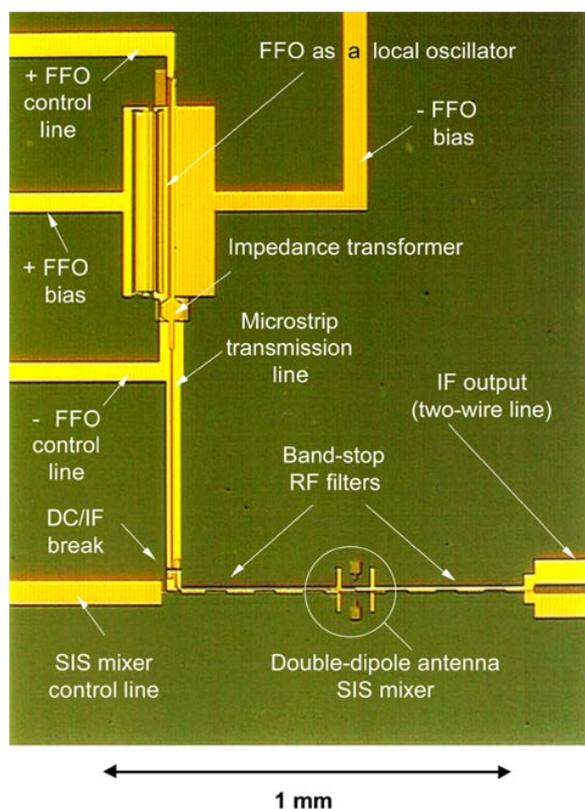
**Figure 7.** Microphotograph of a central part of the silicon chip of sizes 4 mm by 4 mm. All main elements of the integrated receiver are presented; the back reflector is not yet installed on the double-dipole antenna. Some details of wiring and contact pads are out of the field of view, which is about 1 mm by 1.5 mm.
