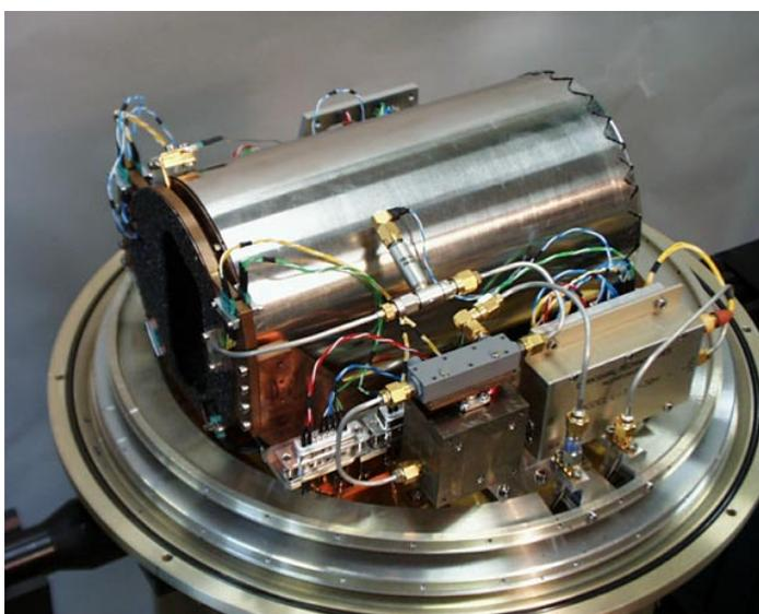
**Figure 16.** Open cryostat with nine-pixel imaging array mounted inside the cylindrical shielding can at 4.2 K. A low noise HEMT IF amplifier with magnetically shielded isolator and directional coupler are in the foreground.
