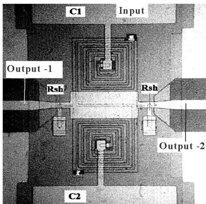
**Figure 18.** Partial view of chip of balanced SQA [32]. Two capacitors  $C_1$  and  $C_2$  and two series input coils (inside holes of the SQUID washer) are tuned at about 4 GHz. The wide strip in the centre is a superconducting control line for magnetic bias of the SQUID. Two outputs, connected to each of two shunted SIS junctions, provide rejection of the common mode. Output filters are out of the field of view.
