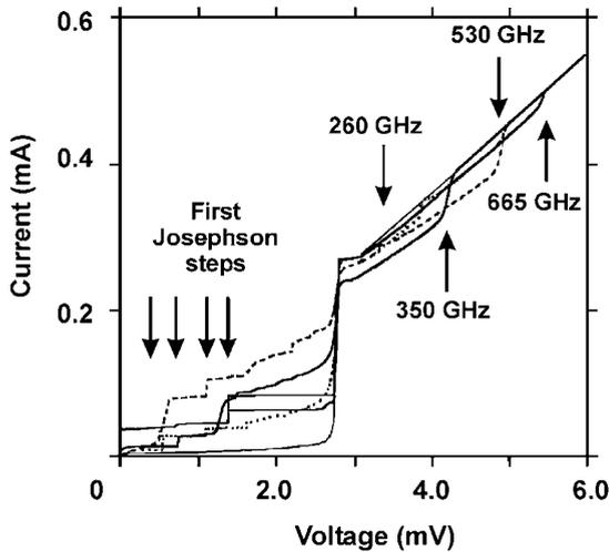
**Figure 2.** IVCs of the SIS detector (wide band design) pumped by an FFO at different frequencies [21]. The arrows are pointing to quasi-particle (tunnel-assisted) steps and first Shapiro steps for frequencies 260, 350, 530 and 665 GHz.
