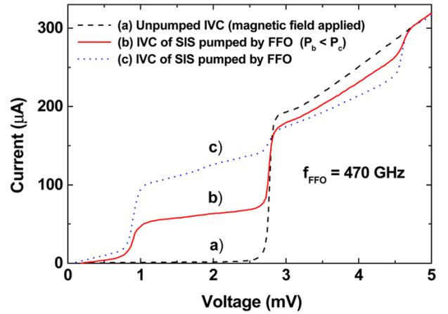
**Figure 3.** IVC of the SIS mixer: a, without FFO pumping; b and c, pumped by the FFO at 470 GHz for two levels of the FFO power (explained in the text) [39]. The ac Josephson effect is suppressed by current through the integrated control line.
