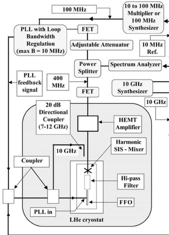
**Figure 4.** Block diagram of the PLL circuit and set-up for linewidth measurement [49]. The central components are the cryogenic chip with the FFO and SIS mixer, the cooled low noise 400 MHz HEMT IF amplifier and the 10 GHz synthesizer, which also provides a 10 MHz reference signal for the spectrum analyser and the PLL phase detector.
