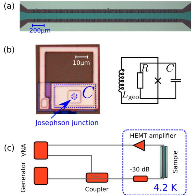
FIG. 2. (a) An image of the rf-SQUID metamaterial showing 54 rf-SQUIDs coupled to a coplanar waveguide. (b) Left: Photo of a single rf-SQUID. Right: Equivalent circuit model of an rf-SQUID (resistively and capacitively shunted Josephson junction model [27]). (c) The experimental setup consisting of a  $^4\text{He}$  cryostat at 4.2 K, a microwave generator (GEN), and vector network analyzer (VNA).
