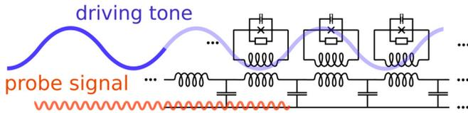
FIG. 1. The main idea: the nonlinear response of the metamaterial to a large-amplitude driving tone (blue) is investigated by a weak probe signal (orange). The response to the weak signal is linear; however, it contains information about the large-amplitude response to the driving tone.
