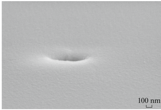
Fig. 5. Test junction based on resist ma-N 2400 with a diameter of 0.4 \mu\text{m} after deposition of the \text{SiO}_2 insulation and “explosive” lithography.
