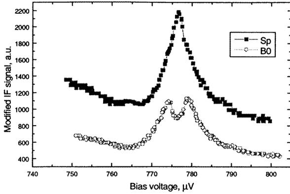
**Figure 4.** Experimental IF output signal (circles) and extracted spectrum (squares).
