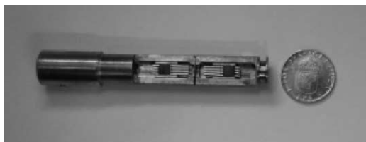
Fig. 3. Photo of a dipstick version of the back-to-back attached receiver and oscillator chips forming a submm-wavelength tester for cryogenic radiating and receiving structures.
